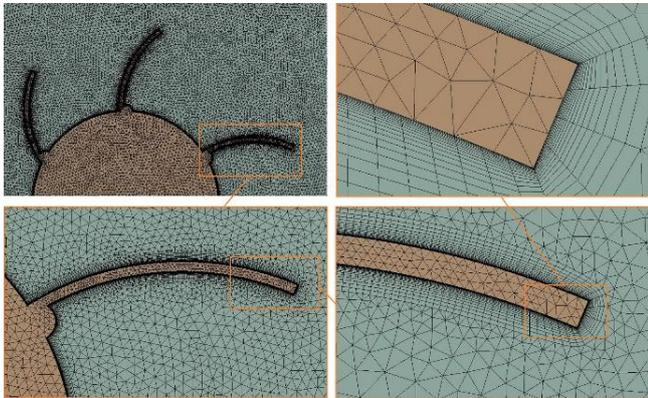
**Fig. 2. Fine mesh around the complex geometry**
