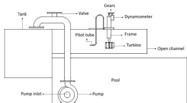
Fig. 1. Schematic side view of the experimental setup
