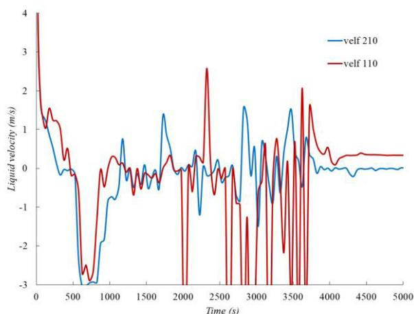
**Fig. 2. Liquid velocity in the hot legs of first and second loops during SB-LOCA with 100 mm break**
