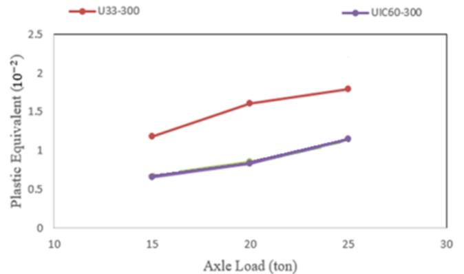
Fig. 7. Result of different plastic deformation by considering the kinematic and isotropic deformation.
