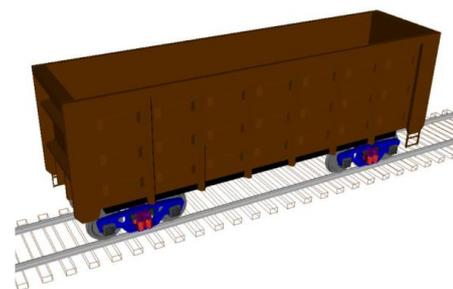
Fig. 1. Model of freight wagon using 18-100 bogie
