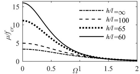
Fig. 1. Homoclinic bifurcation diagram and chaos threshold of the system for different values of size ratio ( $h/l$ )
