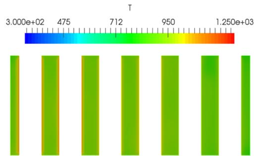
Fig. 6. Temperature distribution around the reactor tubes
