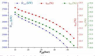
Fig. 5. Effects of the kalian high pressure on the performance of the proposed cycle
