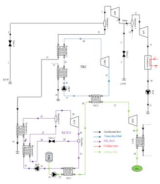
Fig. 1. The new proposed cycle for the power and natural gas production
