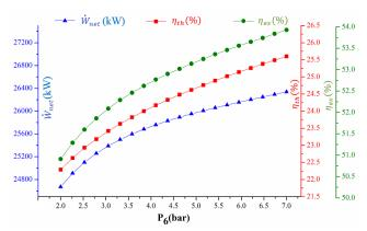
Fig. 3. Effects of the second separator pressure on the performance of the proposed cycle
