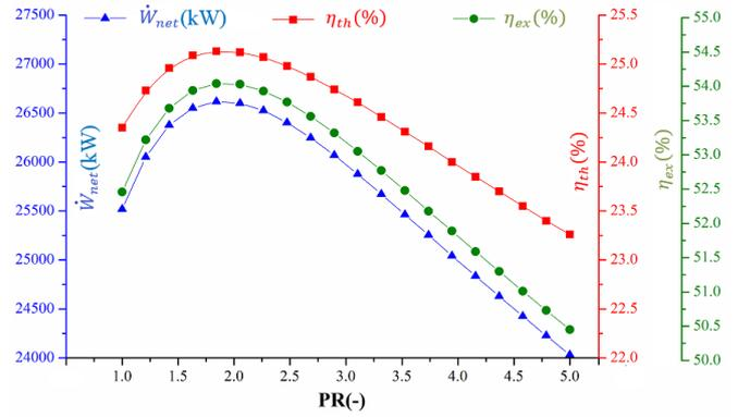
Fig. 4. Effects of the CO<sub>2</sub> cycle pressure ratio on the performance of the proposed cycle
