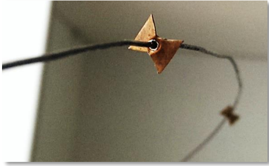
Fig. 2. Butterfly tube insert for using in copper tube.
