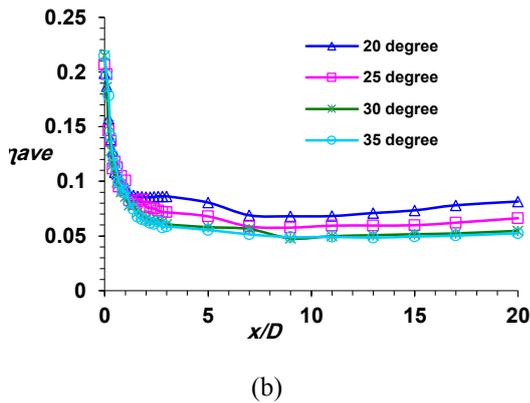
Fig. 2. Comparison of the pulse film cooling effectiveness at different angles and 50 Hz (a): centerline (b): averaged laterally
