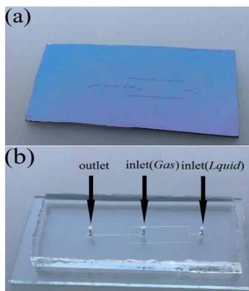
Fig. 1: (a) Photoresist mold (b) PDMS flow-focusing device.
