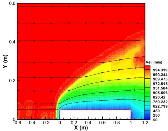
**Fig. 1. The velocity contours of the cylindrical problem**
