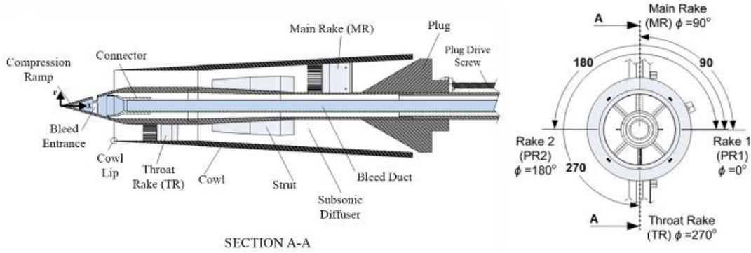
Fig. 2. Schematic view of the intake model and its instrument [1]
