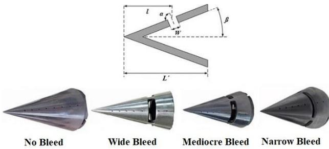
Fig. 3. Spike tip cones used in this study
