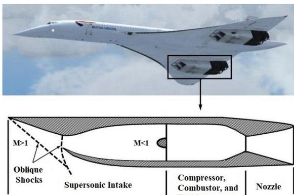
Fig. 1. The engine components in a supersonic airplane
