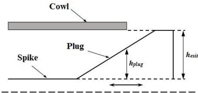
Fig. 4. Parameters used in the definition of EBR
