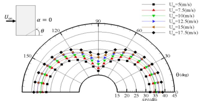
**Fig. 3. Directivity noise patterns for CAARC model on the YZ plane ( $X=0$ ) plane ( $r=2m$ ) and  $\alpha=0$ .**
