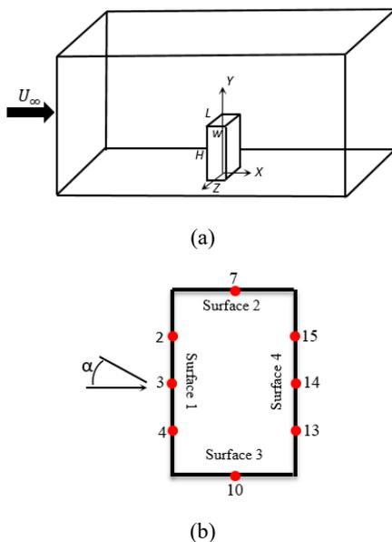
**Fig. 1. (a) Schematic drawing of the model; (b) surface pressure measuring points on the middle height belt.**
