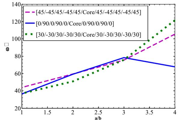
Fig. 3. The effect of panel length to width ratio on the dimensionless natural frequency
