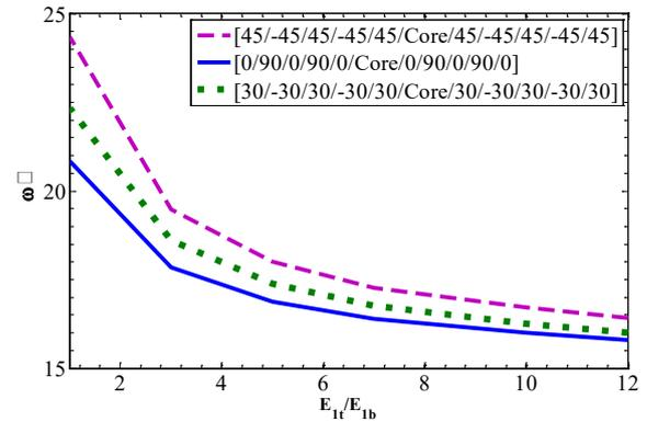
Figure 2. The effect of elastic modulus ratio of the face sheets on the dimensionless natural frequency
