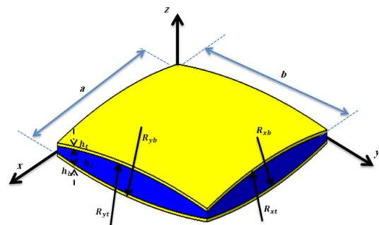
**Fig. 1. The geometry of the studied doubly curved sandwich panel**
