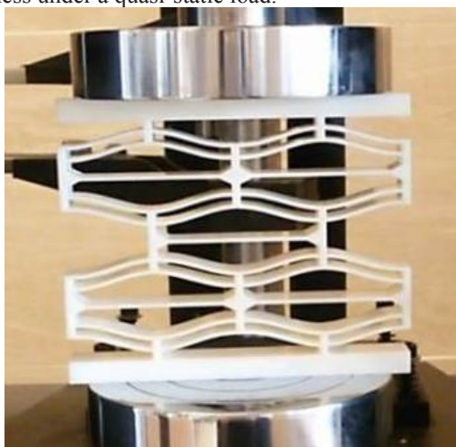
Fig. 1. Negative stiffness honeycomb with constant thickness under a quasi-static load
