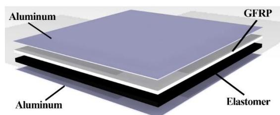
**Fig. 1. The layers' arrangement in the hybrid structure**
