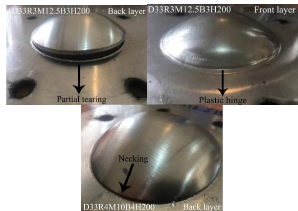
Figure 2. Typical specimens after blast loading
