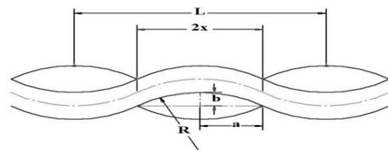
Fig. 1. The schematics of the yarn cross-section
