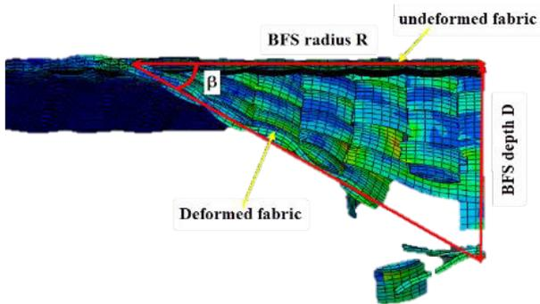
Fig. 4. The illustration of the pyramidal fabric deformation
