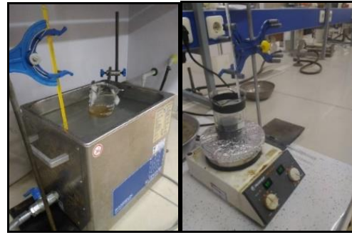
Figure. 1. Ultrasonic bath (right) and magnetic stirrer (left)
