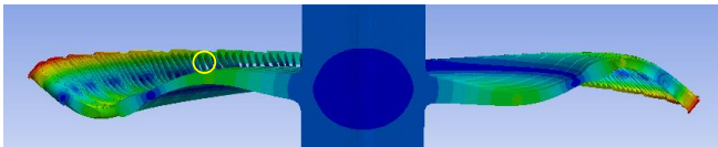
Fig. 2. Shaft-disk-blades system cross section view at the first ND of the 11 th mode; circle shows the position of NES.
