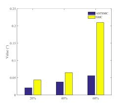
Fig. 4. RMS of tracking error in presence of different disturbances
