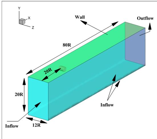
Fig.e 1. Solution domain and applied boundary conditions.
