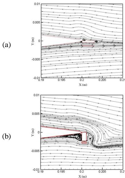
**Figure 3 Flow streamlines of (a) maximum aerodynamic efficiency and (b) maximum lift coefficient**
