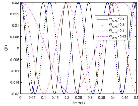
**Figure 5: Comparison of the time response of the nonlinear vibration of pipe conveying fluid made of multilayer composite materials reinforced by graphene platelets for the different graphene weight fractions (pattern V).**
