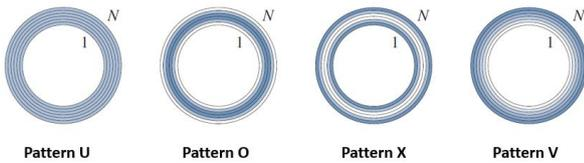
Figure 1: Four different distribution patterns of the graphene platelets along the thickness of the pipe
