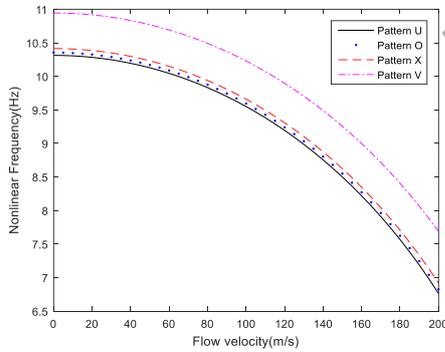
**Figure 4: First nonlinear natural frequency of the graphene reinforced pipe conveying fluid in terms of the fluid velocity for the different graphene distribution patterns**
