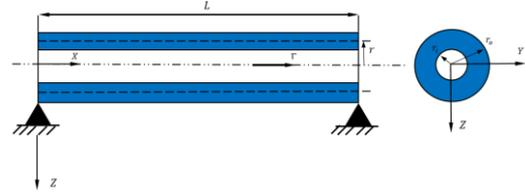
Figure 2: Simply-supported polymer pipe conveying fluid reinforced by graphene platelets
