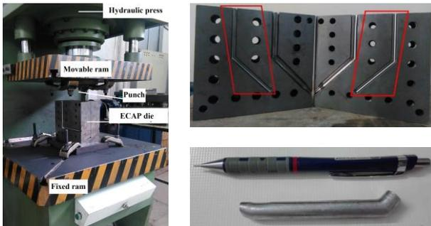
**Fig. 1: The real view of (a) set-up of process and (b) ECAP die and used channel with angle of 135 degree, corner angle of 20 degree and diameter of 10 mm (shown in the red box)**
