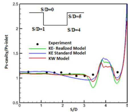
**Figure 2. Comparing non Dimensional static pressure(versus inlet static pressure) for various methods of RANS with experimental data[9]**
