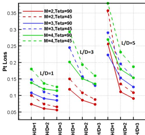
Figure 5. Total pressure loss for various H/D, L/D and Mach numbers at outlet
