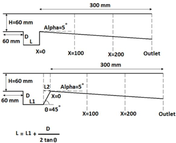
**Figure 1. Schematic representation of geometrical dimensions of combustors in present work**
