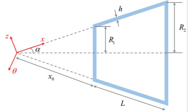
Figure 1. Side view of a truncated conical micro-shell.
