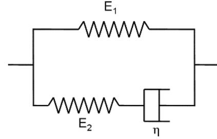
Figure 1. Standard Linear Solid model
