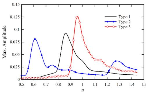
**Figure 5. Maximum amplitude of vibration of a viscoelastic beam's midpoint in terms of external fluid flow velocity**
