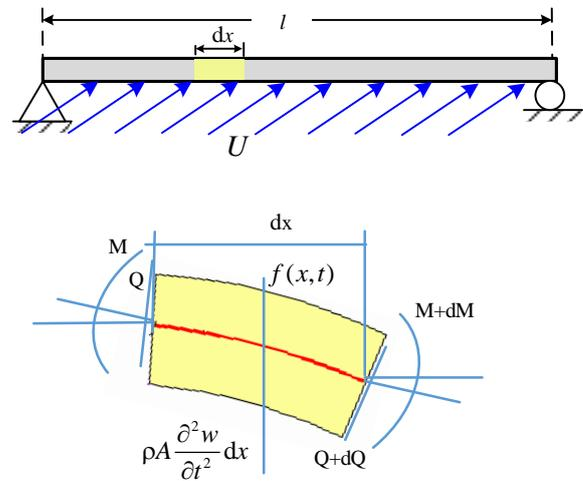
Figure 2. Simply supported viscoelastic beam under the influence of external fluid and a section of the beam
