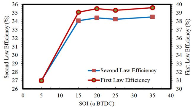
Fig. 3. Effects of the start of injection timing on first and second law Efficiency
