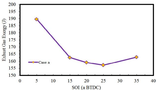
Fig. 2. Effects of the start of injection timing on Exhaust Gas Exergy
