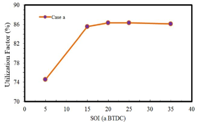
Fig. 4. Effects of the start of injection timing on utilization factor
