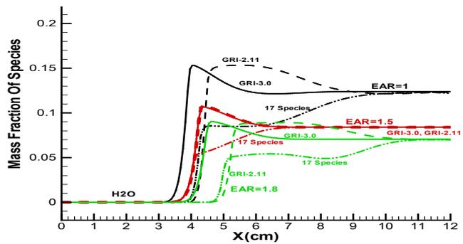
Fig. 6. Diagram of the mass fraction of H<sub>2</sub>O species using the combustion mechanisms GRI-2.11, GRI-3.0 and the 17-species mechanism for different values of the excess air ratio
