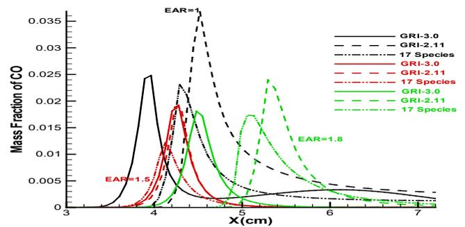
Fig. 8. Diagram of the mass fraction of CO species using the combustion mechanisms GRI-2.11, GRI-3.0 and the 17-species mechanism for different values of the excess air ratio
