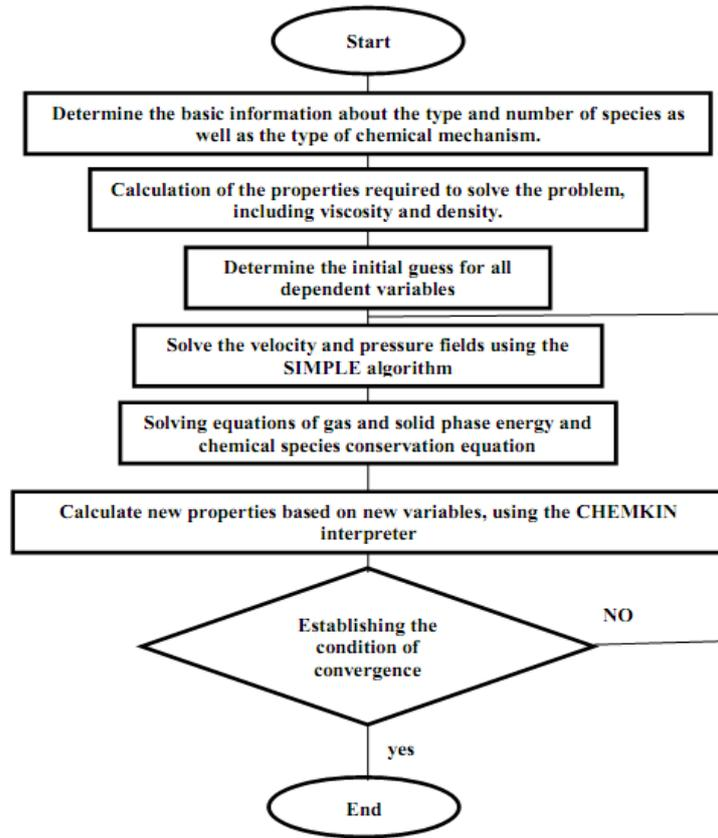
Fig. 2. Flowchart numerical simulation algorithm
