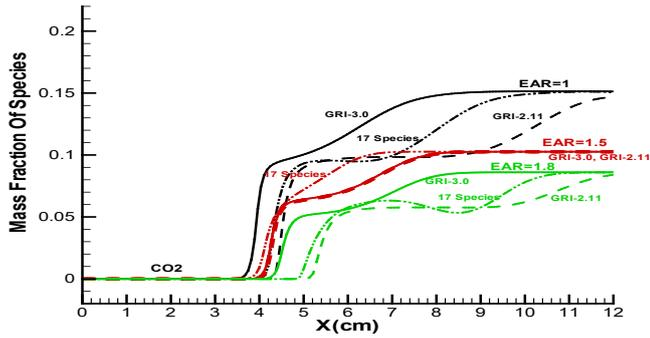
Fig. 5. Diagram of the mass fraction of CO<sub>2</sub> species using the combustion mechanisms GRI-2.11, GRI-3.0 and the 17-species mechanism for different values of the excess air ratio
