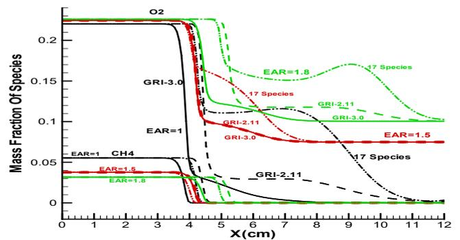
Fig. 4. Diagram of the mass fraction of species using the combustion mechanisms GRI-2.11, GRI-3.0 and the 17-species mechanism for different values of the excess air ratio
