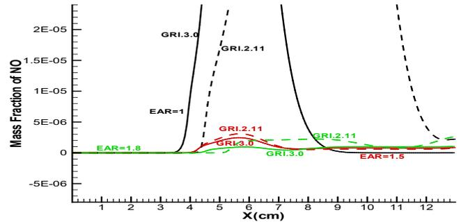
Fig. 7. Diagram of the mass fraction of NO species using the combustion mechanisms GRI-2.11, GRI-3.0 for different values of the excess air ratio
