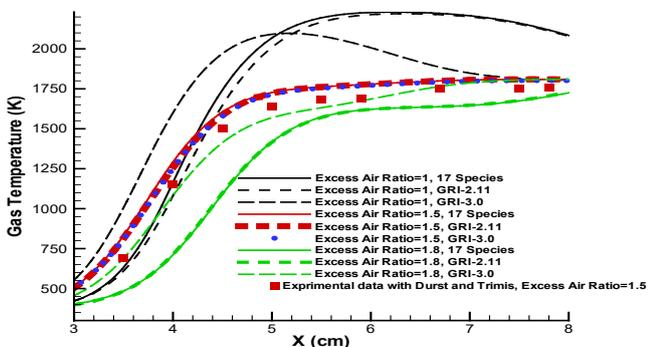
Fig. 3. Gas temperature diagram using the GRI-3.0, GRI-2.11 and 17-species mechanisms for different values of the excess air ratio [6]
