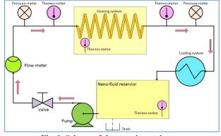
Fig. 1. Scheme of the experimental setup
