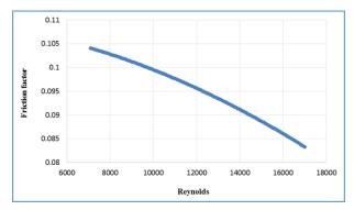
Fig. 3. The variation of friction factor versus *Re*
