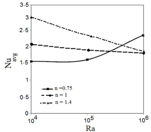
Fig. 5. Variations of average Nusselt in the Rayleigh numbers for different power indexes in the presence of magnetic field
