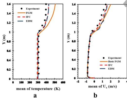
Figure 2. a) Temperature and b) velocity at the doorway
