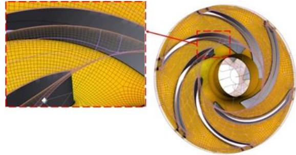
**Figure 1. Pump impeller meshing**
