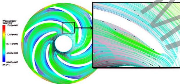
Figure 5. flow separation at inlet pressure of 20 kPa
