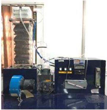
Figure 1. real shape of laboratory cooling tower
