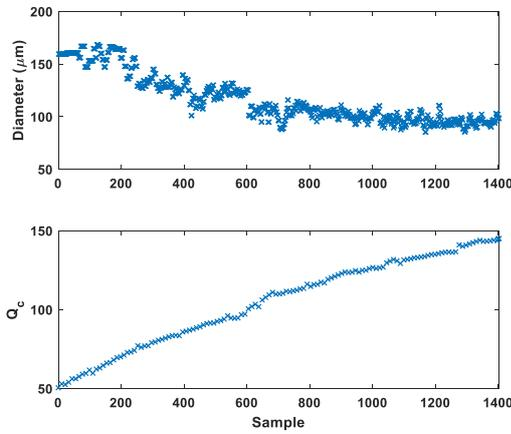
Fig. 2. Diagram for the desired diameter of 100 versus time-step, and diagram of the continuous flow (oil) versus time-step (control command) (RSME=5.27)
