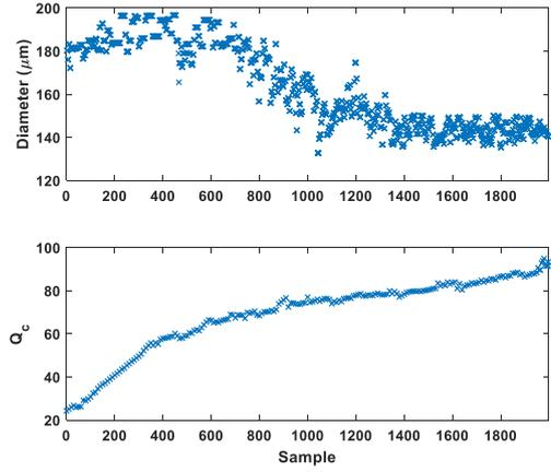
Fig. 3. Diagram for the desired diameter of 140 versus time-step, and diagram of the continuous flow (oil) versus time-step (control command) (RSME=3.4)
