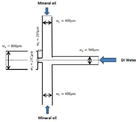
Fig. 1. Dimensions of the microchannel built to control the size of generated droplets
