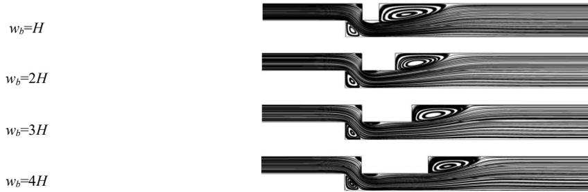
Fig. 2. Streamlines ( $\phi=0.03$ ,  $Re=100$ ,  $h_b=H$ ).
