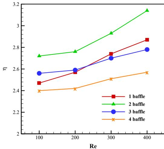
Fig. 4. Performance evaluation index based on the number of baffle for various the nanoparticles volume fraction ( $h_b=H, w_b=H, \phi=0.01$ ).
