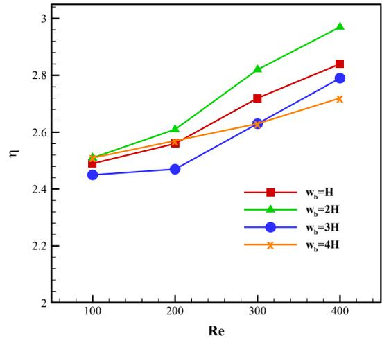
Fig. 3. Performance evaluation index based on the width of baffle ( $h_b=H$ ,  $\phi=0.02$ ).
