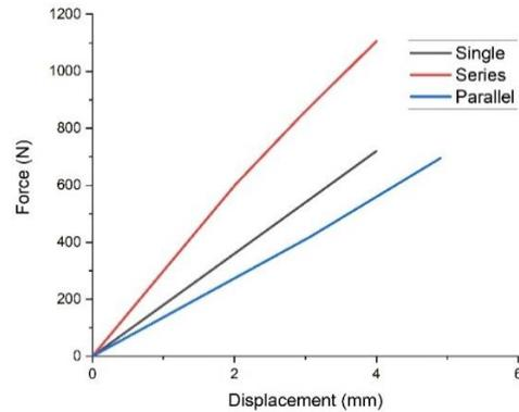
Figure 3. Force-displacement diagram for egg box cores with doubled thicknesses under compression
