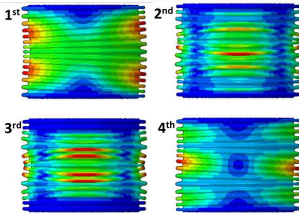
Fig. 2. Four modes of buckling in 15 convolutions bellows
