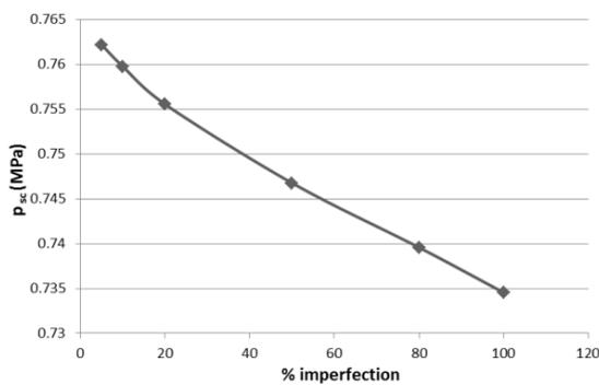
Fig. 5. P<sub>sc</sub> - % imperfection in 15 convolution bellows
