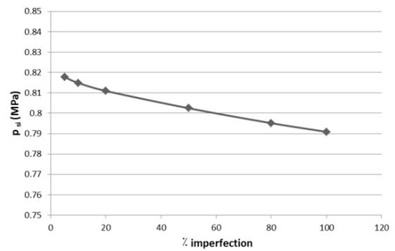
Fig. 4. P<sub>si</sub> - % imperfection in 10 convolution bellows
