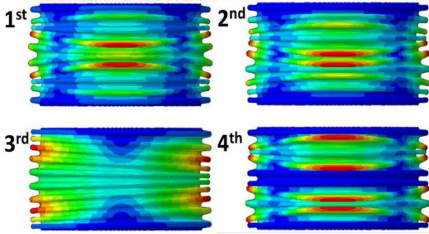
Fig. 1. Four modes of buckling in 10 convolution bellows
