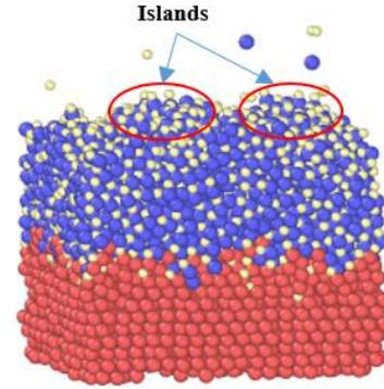
Fig. 3. Snapshot of the deposition process at 3466 ps
