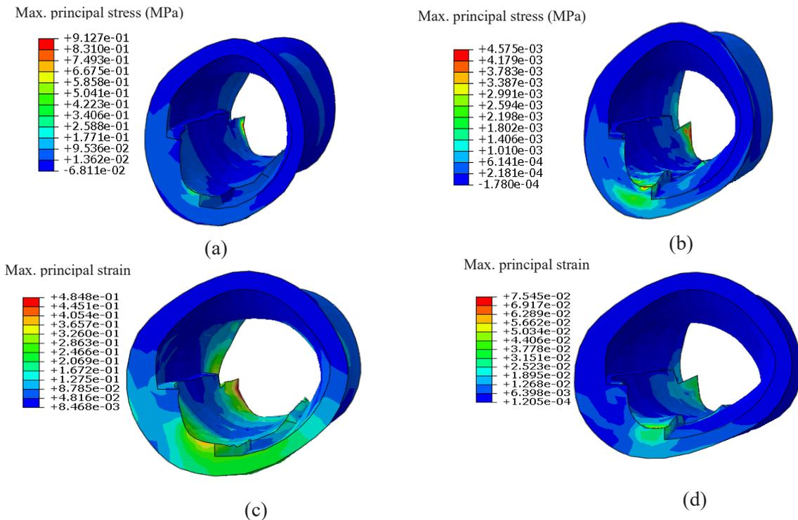
**Fig. 2. (a) The stress of the artery after the artery expansion (b) The stress of the artery after the artery unloading (c) The strain of the artery after the artery expansion (d) The strain of the artery after the artery unloading**
