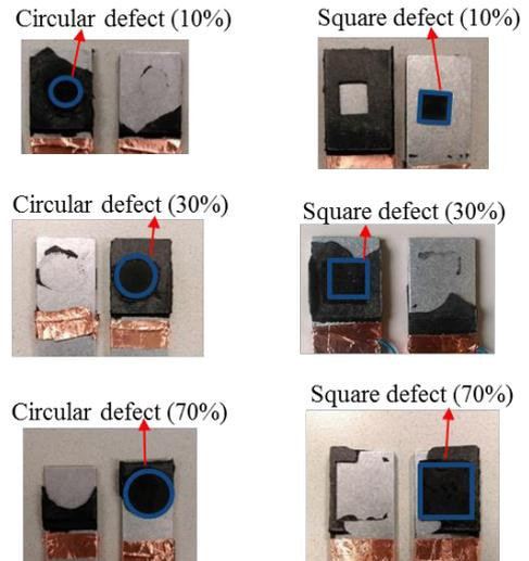
Fig. 3. Fracture surface of defective adhesive joint
