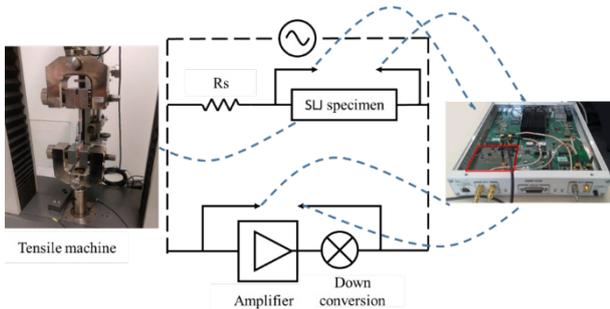
Fig. 2. Electrical measurement setup during the tensile test
