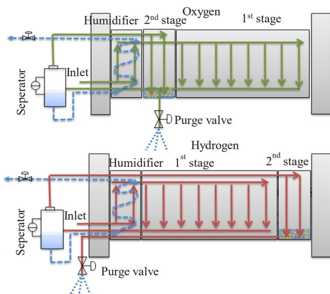
Fig. 1. Schematic diagram of designed fuel cell stack
