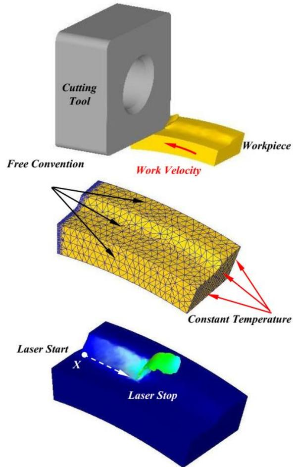
Fig.2. Applying of boundary conditions and laser heat source on the work piece in the finite element model.
