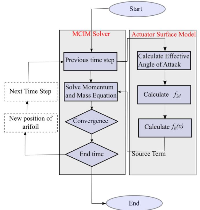
Figure 1. Process diagram of the Flow solver (combination of MCIM solver and AS).
