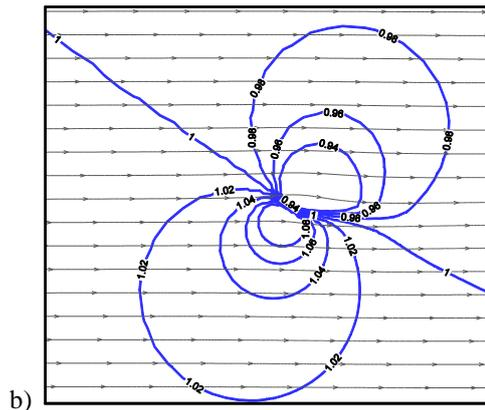
Figure 5. Streamlines and pressure contours with a) Full-CFD and b) CFD-AS; NACA0015,  $Re = 1100$ , Angle of attack of 8 deg.
