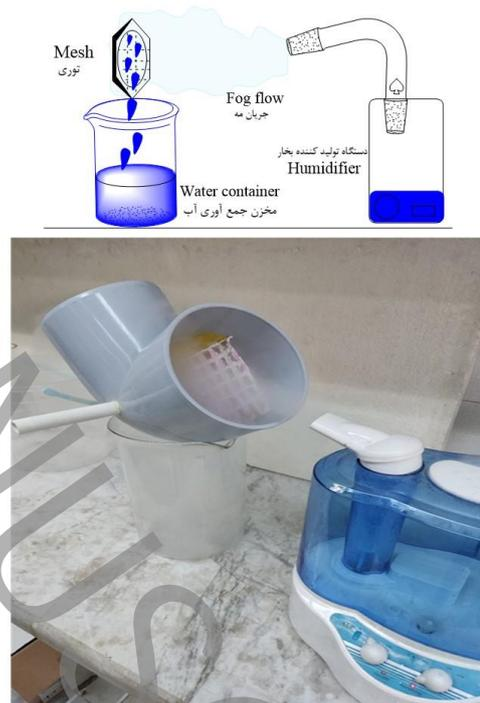
**Fig. 1 Experimental setup. Upper picture: Schematic setup. Lower picture: Real setup**
