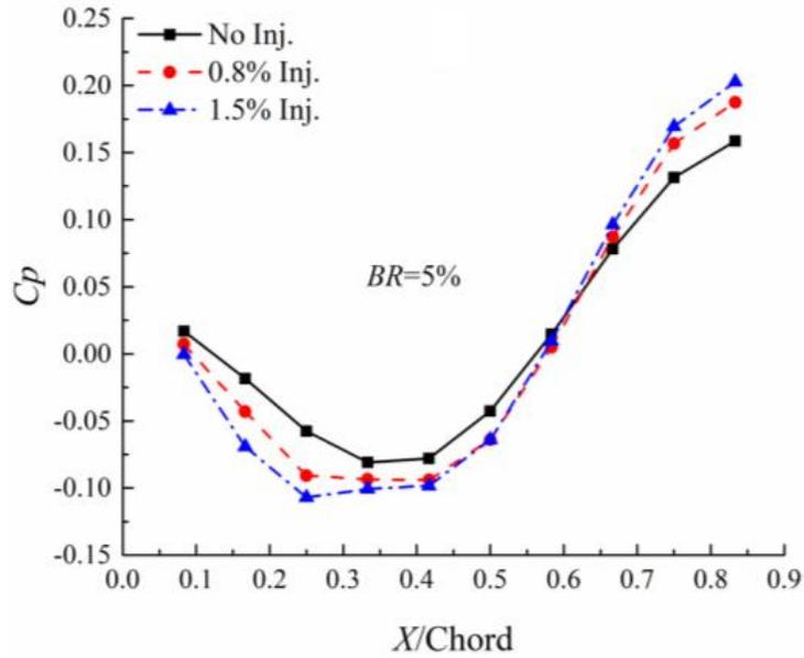
Fig. 3. Static pressure along the blade chord
