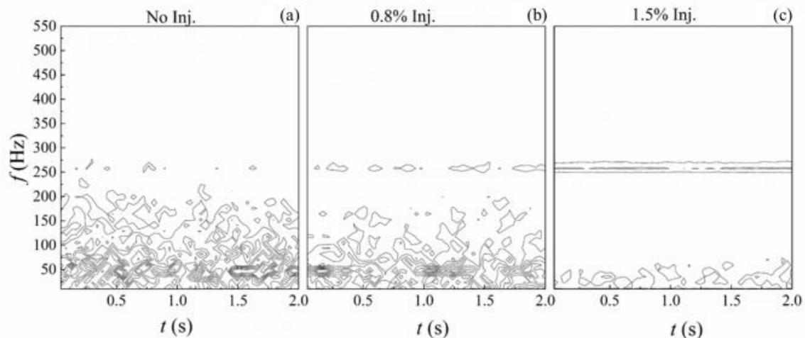
Fig. 5. STFT analysis of static pressure signals, BR=15%
