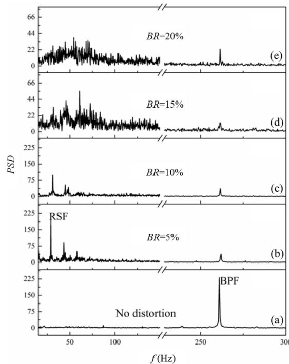
Fig. 2. Frequency spectrums for different distortion cases
