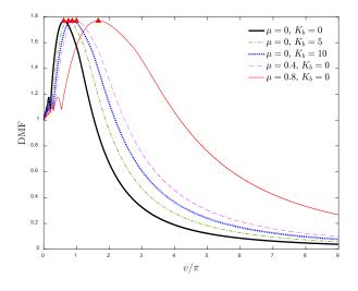
Fig. 1. Dynamic magnification coefficient of system based on dimensionless velocity for various strain gradient parameters and foundation stiffness α=0, γ=0
