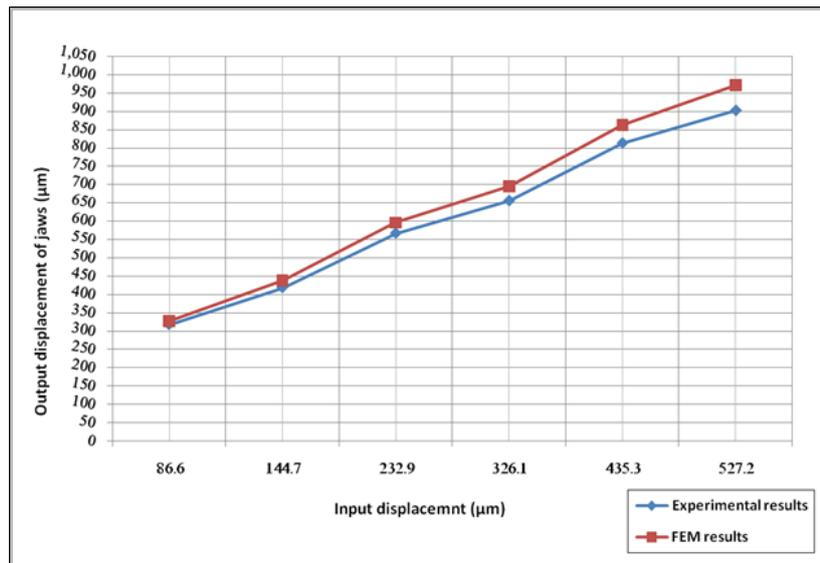
Fig. 4. Variation of the output displacement for the applied input displacement
